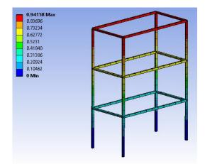
(d). Deformation of fixed base building at 20 s.
