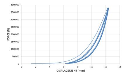
Fig. 4(b). Force verses displacement graph of RTI-5.
