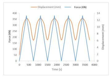
Fig. 4(a). Displacement verses time graph for RTI-5.
