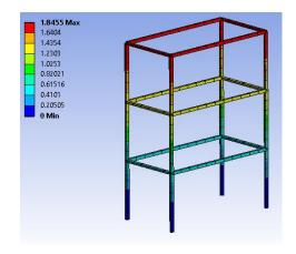
(b). Deformation of fixed base building at 10 s.
