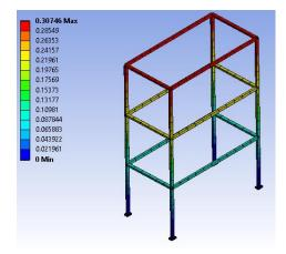
(b). Deformation of base isolated building with RTI at 10 s.
