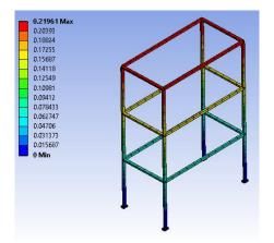
(c). Deformation of base isolated building with RTI at 15 s.
