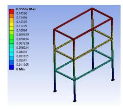
(d). Deformation of base isolated building with RTI at 20 s.
