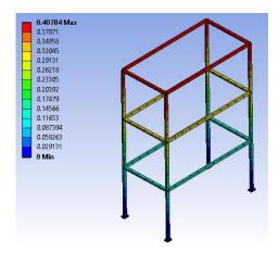
(a). Deformation of base isolated building with RTI at 5 s.
