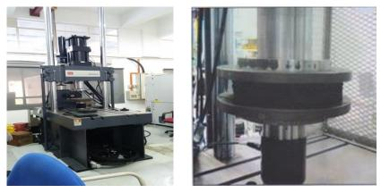
(a) Servo Hydraulic MTS322. (b) Sample under compression.Fig. 3. Overview of test setup.
