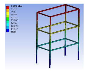
(c). Deformation of fixed base building at 15 s.
