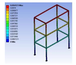
(e). Deformation of base isolated building with RTI at 25 s.
