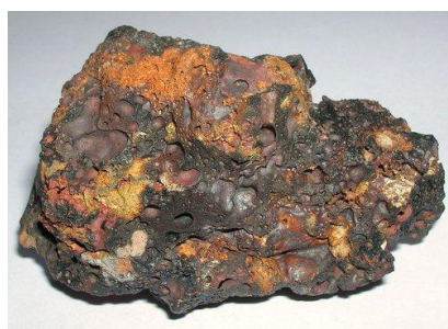
Figure 1: Slag as a by-product from steel making furnace [2]
