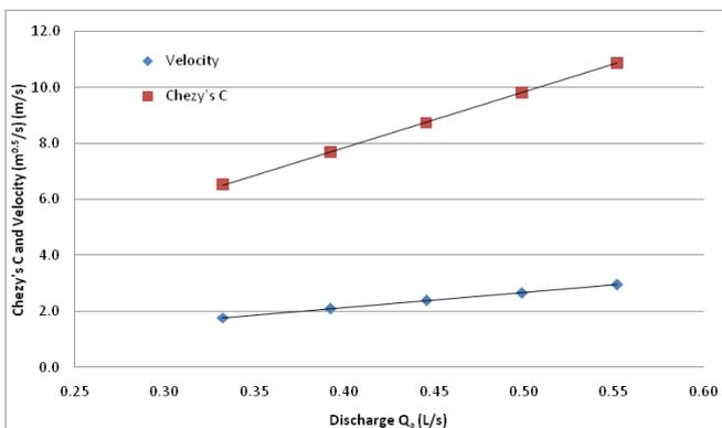
**Figure 7:** Variation of velocity components and discharge The velocity components are highly dependent on discharge and when discharge increases, velocity increases, thereby reducing the friction that is experienced in the channel. However as the aggregate sizes increases, Chezy's  $C$  decreases. This is evidenced in Figure 8.
