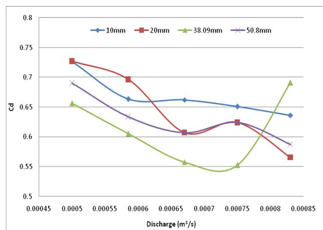
**Figure 3:** Graph showing discharge coefficient values for different aggregate sizes
