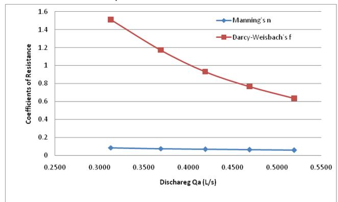
**Figure 5:** Graph of resistance against discharge in an open channel
