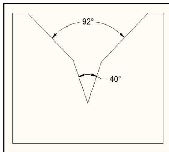
**Figure 2:** Typical Cross section of compound weirs [19].
