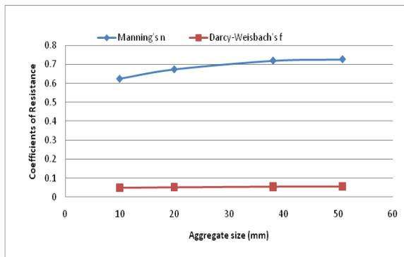
**Figure 4:** Graph of resistance coefficients against aggregate size.
