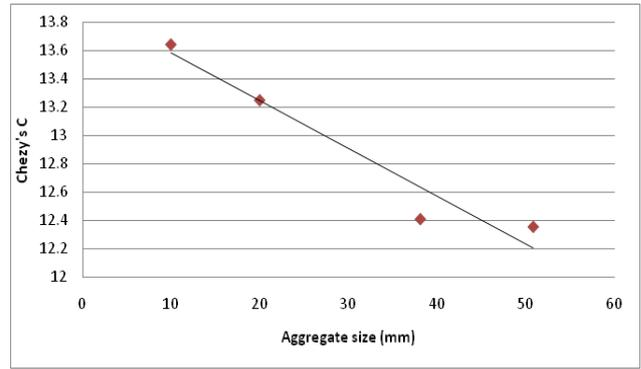
**Figure 8:** Relationship of Chezy's  $C$  and aggregate size A comparison of figure 8 and figure 9 will show that Manning's  $n$  and Darcy Weisbach's  $f$  are inversely proportional to Chezy's  $C$ .
