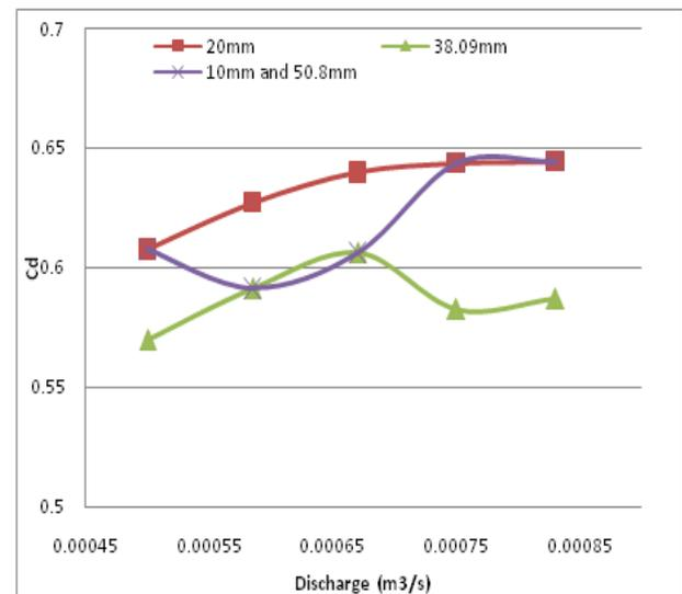
**Figure 2:** Graph showing discharge coefficient values for different aggregate sizes
