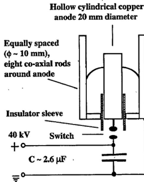
FIGURE 3.A schematic of Imperial College Plasma focus machine [15].
