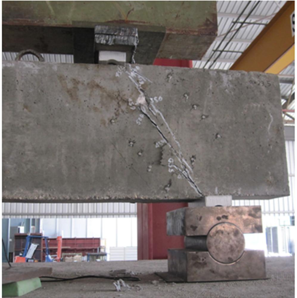
**Fig 6. Typical crack pattern of RC deep beam.**
