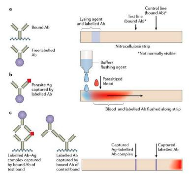
**Figure 7.** Schematic of the lateral flow strip to diagnose Malaria. (top) Layout of the strip, (middle) Flushing agent is added to help flush parasitized blood along the strip, and (bottom) visible lines indicate presence of antigens in the parasitized blood. Reproduced with permission [89].
