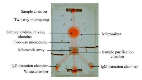
Figure 6. The magnetic bead-based microfluidic chip measures 53 mm  $\times$  37 mm. Reproduced with permission [72].
