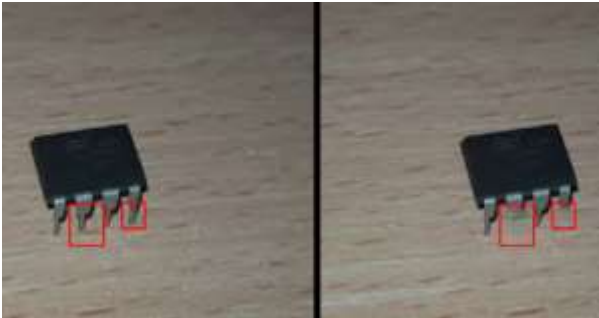
Figure 3a. Pins 2 and 4 are damaged
