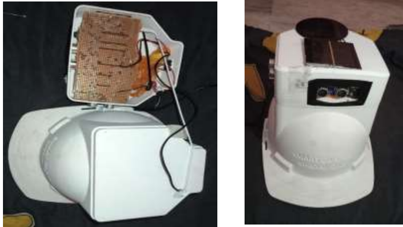
Figure 4. Smart Cap 3D Print Model- internal and external view of prototype
