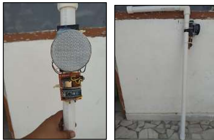
Fig. 6. Smart Cane – sensors and prototype view
