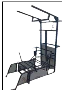
Figure 1. Frame of solar wheelchair
