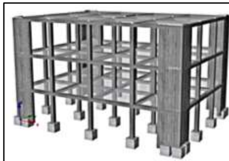
Figure 1. Conceptual of a low-rise reinforced concrete frame integrated with bio-based high-damping composite components as supplementary structural elements (Fuentes & Baez, 2023).
