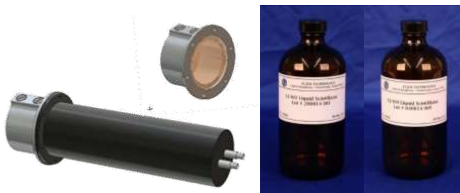
Figure 3 Liquid scintillators: NE-213, EJ-301, EJ-309 liquid scintillator
