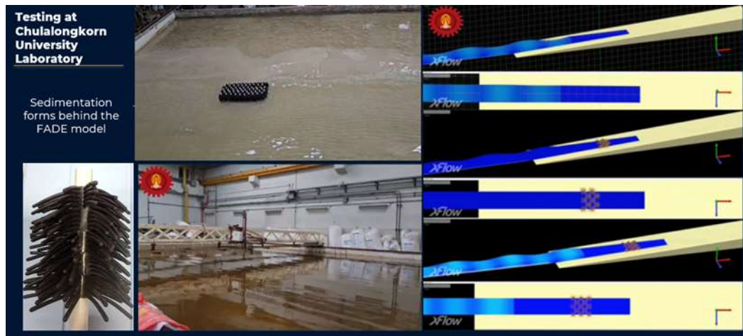
Figure 3. Laboratory testing and CFD simulation of FADS
