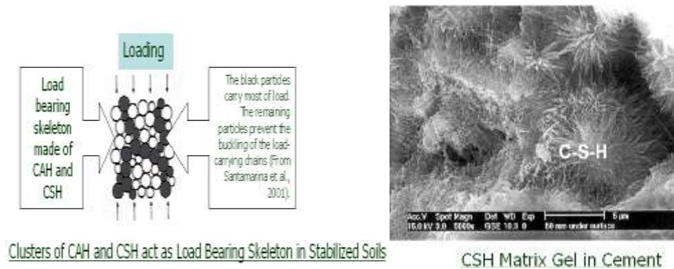
Figure 1. Stiff mechanism resistance within its mass in stabilized soil (Hafez, 2007)
