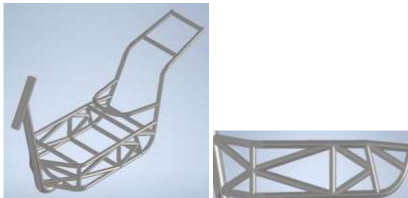
Figure 7. Isometric and side view of chassis design 5.
