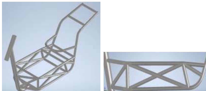
Figure 4. Isometric and side view of chassis design 2.
