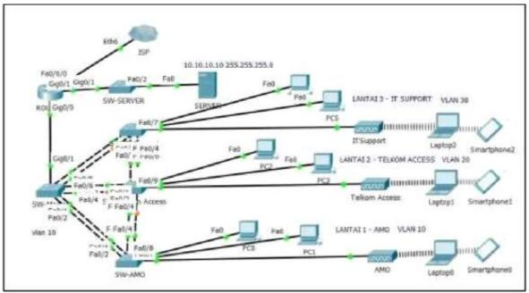
Figure 2. PT. Telkom Network Topology with VLAN-based STP
