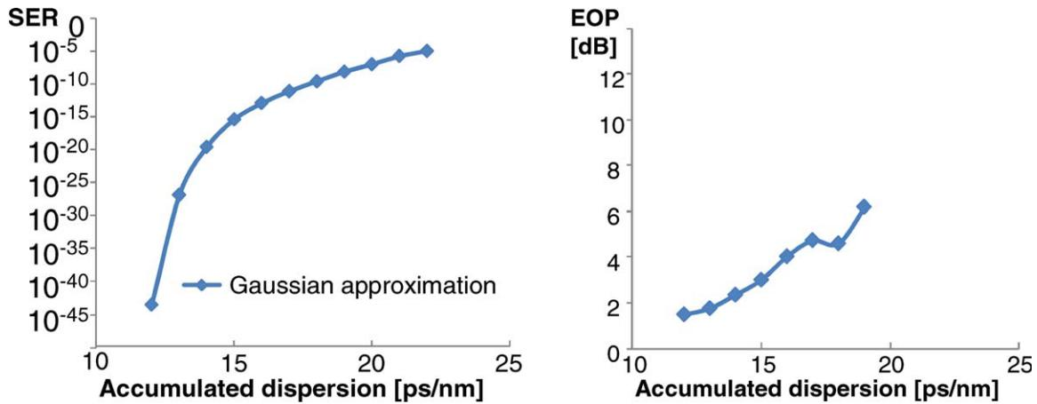
**Figure 8** 16-QAM 100 Gbit/s signal quality estimation in the presence of chromatic dispersion. [Color figure can be viewed in the online issue, which is available at [wileyonlinelibrary.com](http://wileyonlinelibrary.com)]
