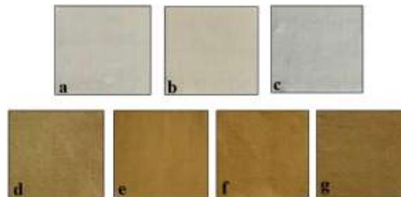
Figure 1. Representative images for plain cotton fabric (a), cotton fabric soaked in *A. malaccensis* leaf extract (b) and 1000 mM CuSO<sub>4</sub> (c), and CNCFs using 100 mM (d), 200 mM (e), 500 mM (f), 1000 mM (g) of CuSO<sub>4</sub> as a precursor during *in-situ* syntheses of nanoparticles.
