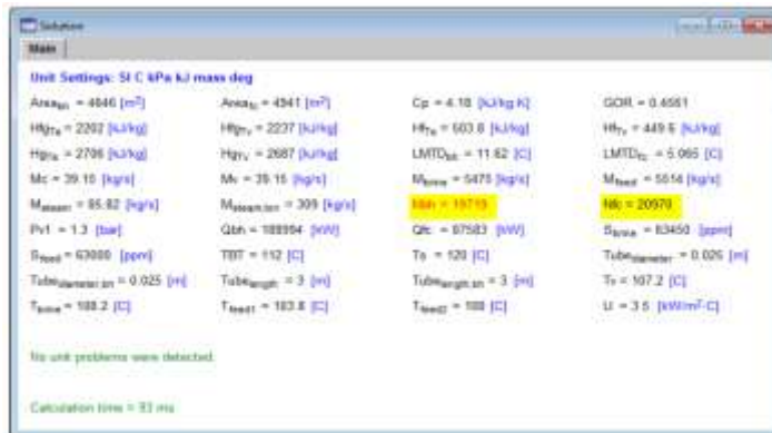
Figure 6. The results for the brine heater and flash chamber using EES software.
