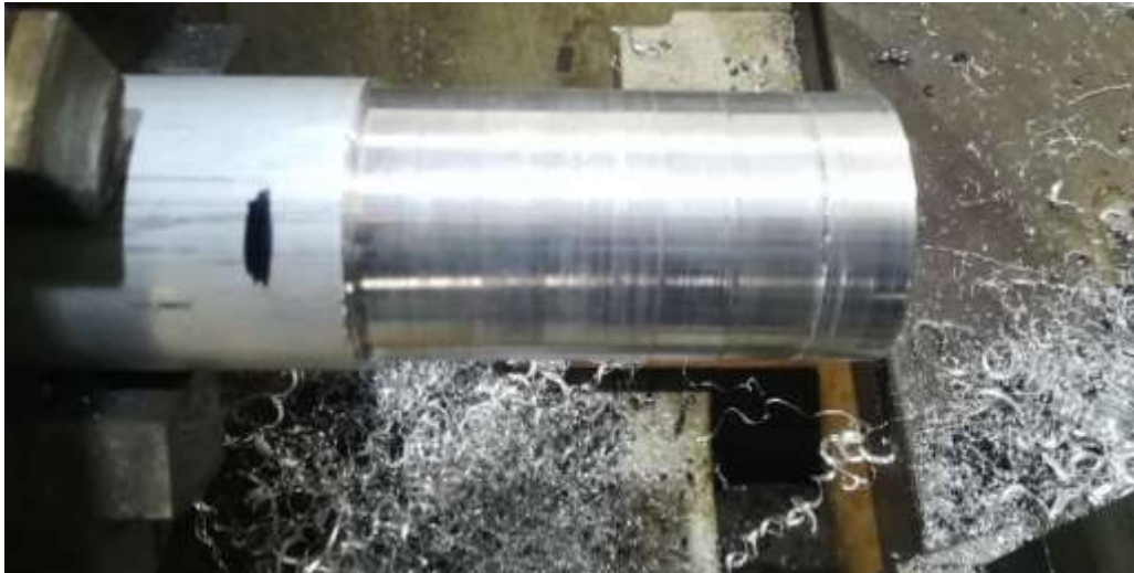
Figure 4. Dry cutting of aluminium in a lathe machine
