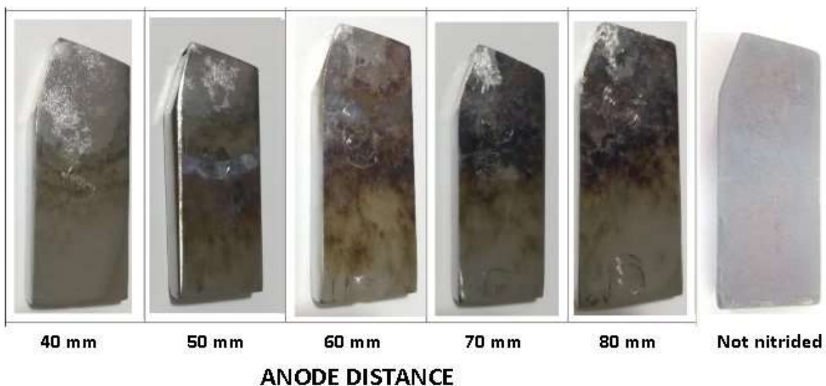
Figure 5. Visual inspection of the pitted tool end
