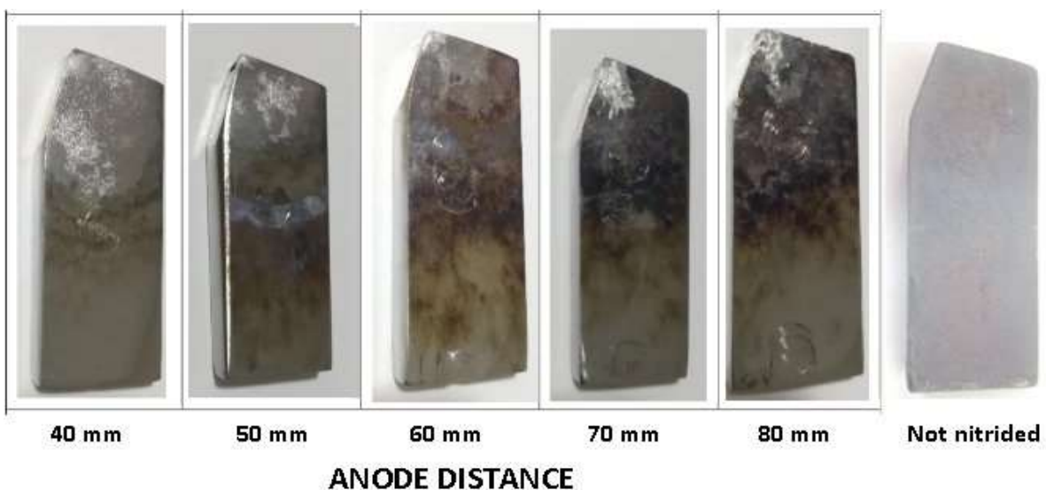
Figure 5. Visual inspection of the pitted tool end
