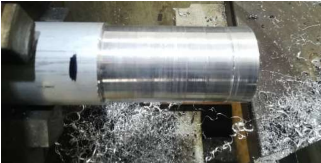
Figure 4. Dry cutting of aluminium in a lathe machine
