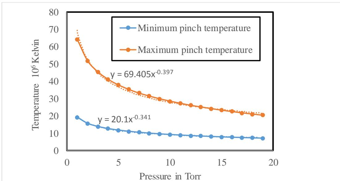
Figure 3. Computed Plasma pinch temperature versus pressure.
