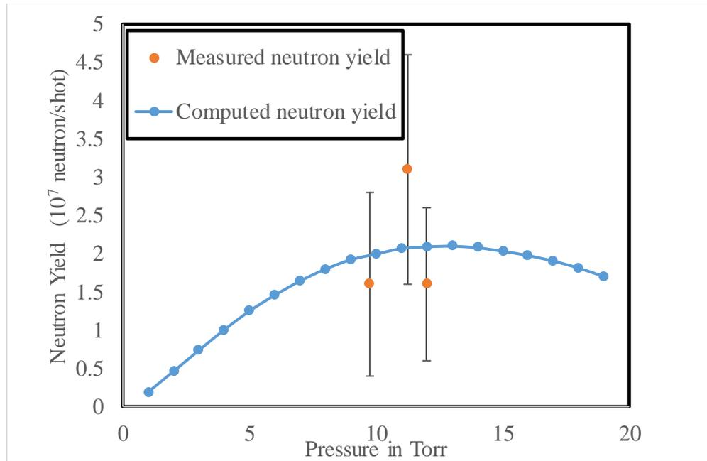
Figure 4. Computed and measured neutron yield versus pressure.
