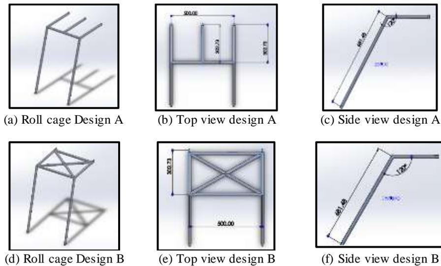
Figure 1. Design A and B
