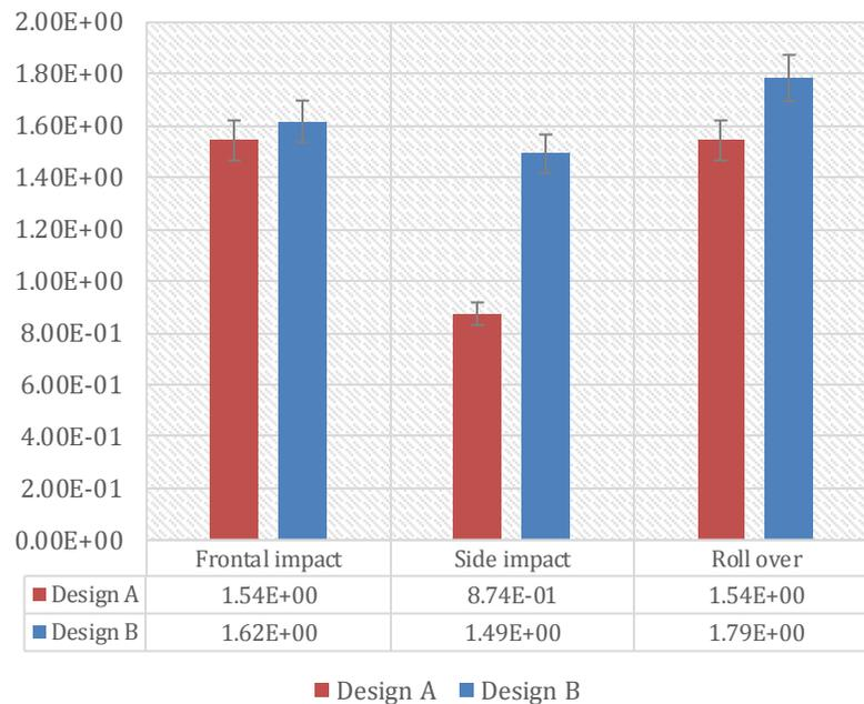
Figure 2. Comparison of factor of safety against the impact test on design A and B.
