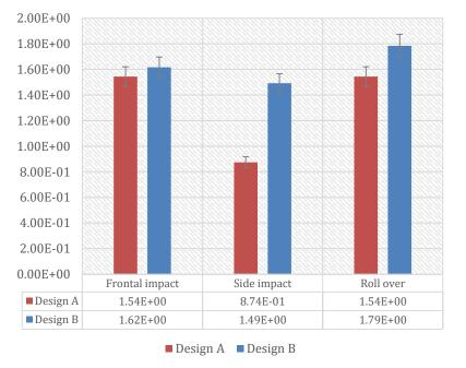
Figure 1. Comparison of factor of safety against the impact test on design A and B.
