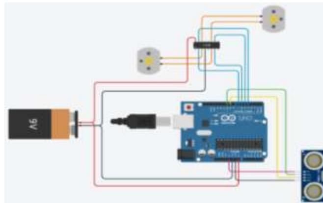
Figure 2: Obstacle avoiding robot circuit diagram
