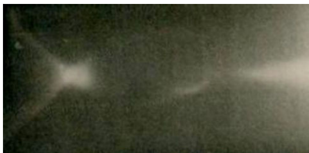
Fig. 1 Streak photograph of UMDPF1. The axis of symmetry is the horizontal line across the vertical middle of the photograph. Vertical scale is distance, being 25 mm across the whole vertical length of the photograph. Horizontal scale is time, being 300 ns across the horizontal length of the photograph
