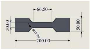
Figure 1. Dimensions of the specimen for tensile test
