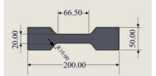
Figure 1. Dimensions of the specimen for tensile test
