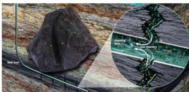
Figure 2: Fracking tight shall formation (Anttu Lein, 2014).
