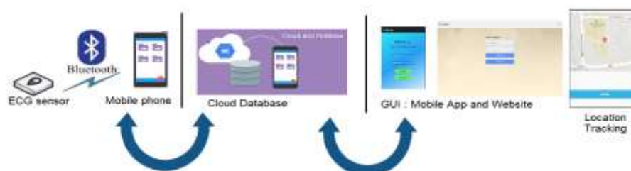
Figure 4. Architecture of Cloud based Heartbeat Monitoring System with Location Tracking
