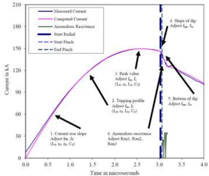
Figure 2. The 6 –point fitting of computed current trace obtained from shot number 11 of INTI International University Plasma focus machine operated at 12 kV, 0.5 Torr in nitrogen gas. The fitting uses Lee Model 6-phase code (Singh et al., 2018)
