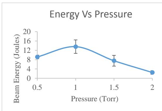
Figure 3. The beam energy of 360 shots taken versus the gas pressure
