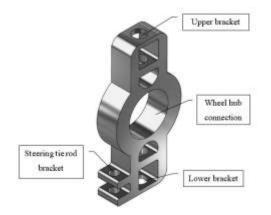
Figure 1. Design of the upright structure
