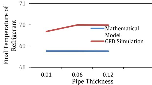
Figure 1. Final temperature of refrigerant vs pipe thickness: comparison of mathematical model and CFD simulation
