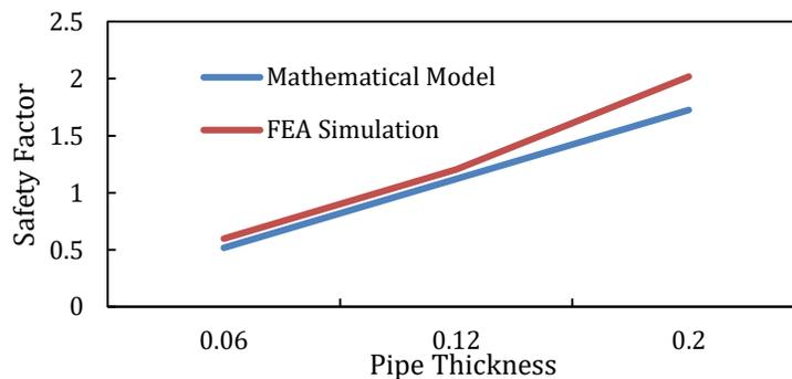
Figure 2. Safety factor against pipe thickness: comparison between mathematical model and FEA simulation
