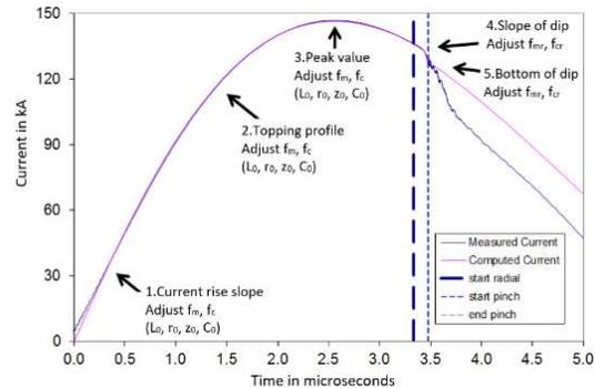
Fig. 3. The 5 phase computed current waveform compared to the corresponding waveform measured from INTI PF operated at 2.0 Torr neon.
