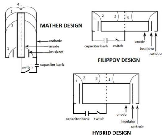
Fig. 1. Mather, Filippov and Hybrid Type Dense Plasma Focus devices schematic drawing.
