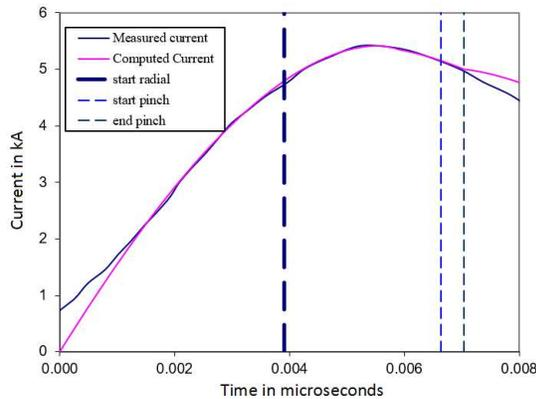
Fig. 7. Measured current waveform of the Nano Focus at 6.5 kV, 2.25 Torr hydrogen gas compared with the fitted current from Lee Model 5-phase code. Note the measured current was obtained from Fig. 4, page 3 of [23].
