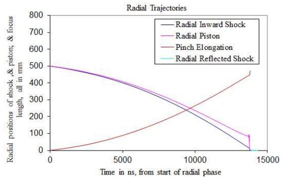
Fig. 6. Radial trajectory of Filippov PF3 according to the Lee Model 5-phase code taken from the same numerical shot as Fig. 5.
