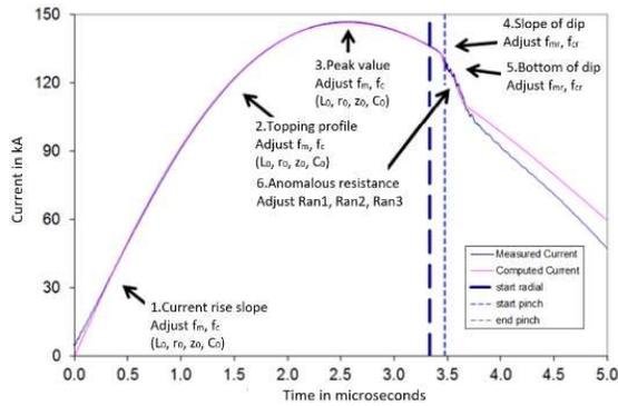
Fig. 4. The 6 phase computed current waveform fitted to the current waveform measured from INTI PF fired at 2.0 Torr in neon.
