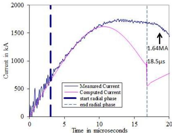
Fig.5. Measured current trace of Filippov PF3 Plasma Focus at 9 kV, 1.5 Torr neon gas compared with Lee Model 5-phase code computed current waveform. Note that the digital waveform for shot 4102 obtained on 3/5/2011 from Mitrofanov Konstantin and Krause Slava authors of [22]).
