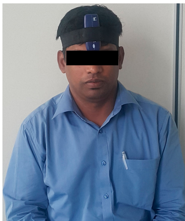
Figure 4. Accelerometer attached to the subject's forehead.
