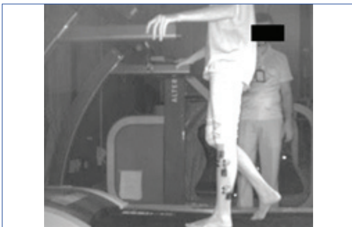
[Table/Fig-4]: Participant with wireless sEMG for testing peroneus longus muscle activation in stance phase of gait.
