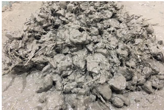
Figure 10: Presence of kenaf fibres produced agglomeration of cement paste, fibres and aggregate particles, affecting the aggregate orientation and void distribution.
