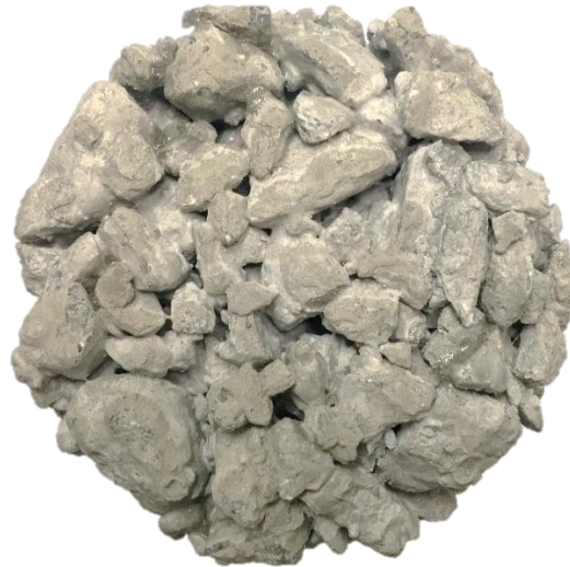
Figure 1: Texture of pervious concrete, containing large amount of voids to allow water permeability
