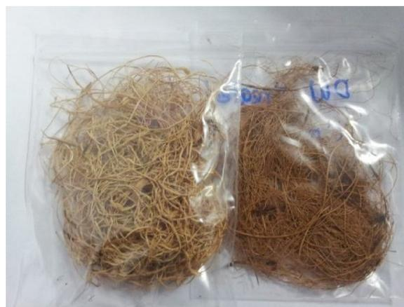
Fig. 2. The coconut fibres (CF, on the right) and oil palm fibres (OPF, on the left) used.
