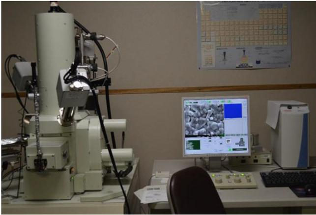
Fig. 3. Overview of the EPMA setup.
