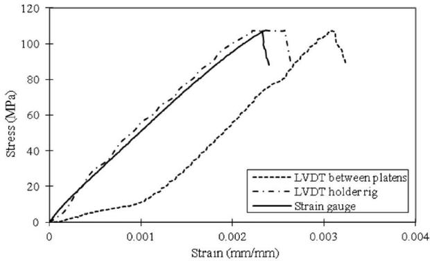
all of the stress-strain curves obtained by LVDT between machine platens.
