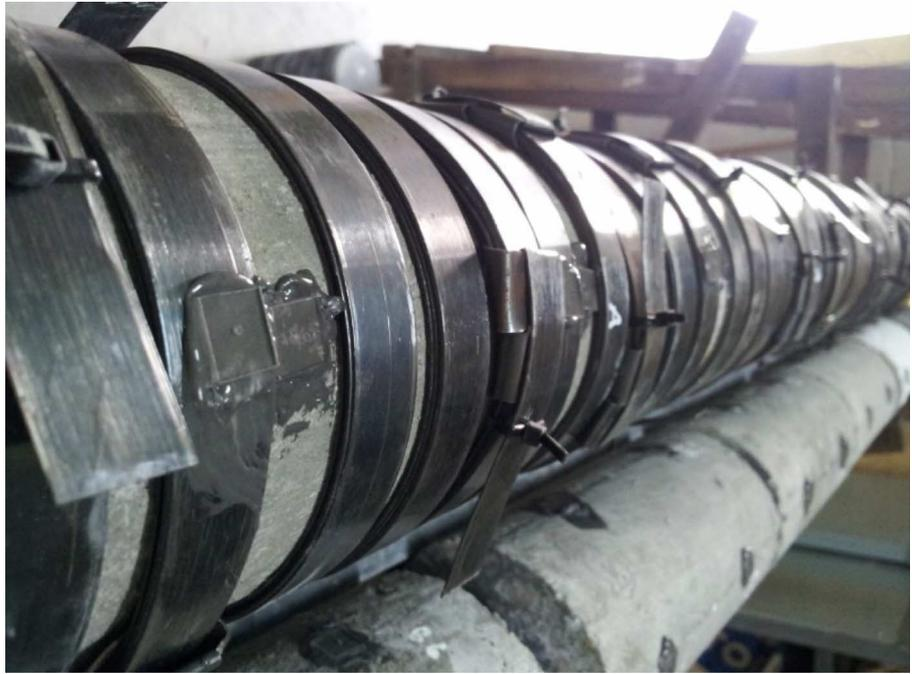
beginning to failure under action of loading. It is quite a challenge to derive the complete stress–strain curve under uniaxial compression because of two reasons: machine–specimen interaction and difficulty in measuring the actual concrete strains from the concrete specimen, especially upon reaching the ultimate compressive strength of the specimen.
