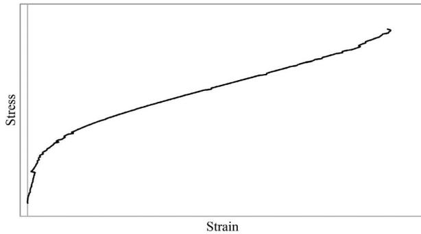
of loaded concrete specimens dropped by more than 50 % of its ultimate compressive strength. In some cases, the tests were stopped once erratic deformation was observed. Normally, erratic deformation happened in the post-peak region. Because such deformation does not represent the aspect of stress–strain behavior, the results were not counted. Some examples of erratic deformation obtained during the load test are shown in **Fig. 6**.
