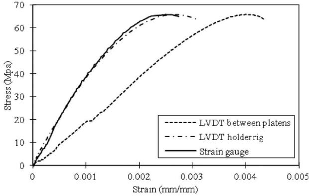
**FIG. 10** Stress-strain curves from various measurement instruments (unconfined concrete specimen of compressive strength 110 MPa).
