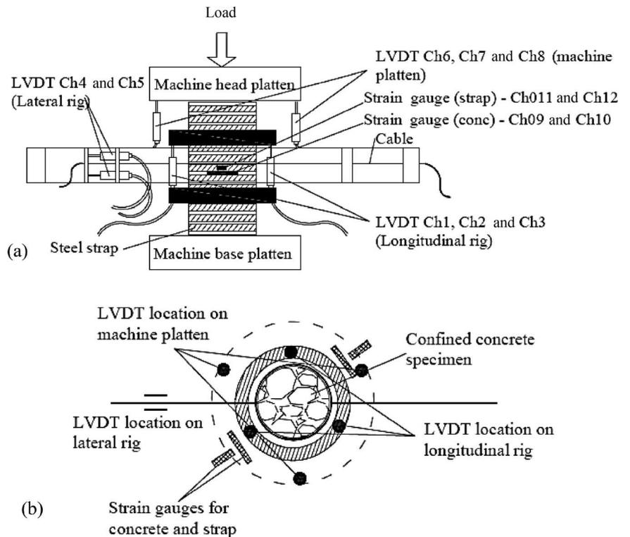
**FIG. 5** Loading pattern for uniaxial monotonic loading test.
