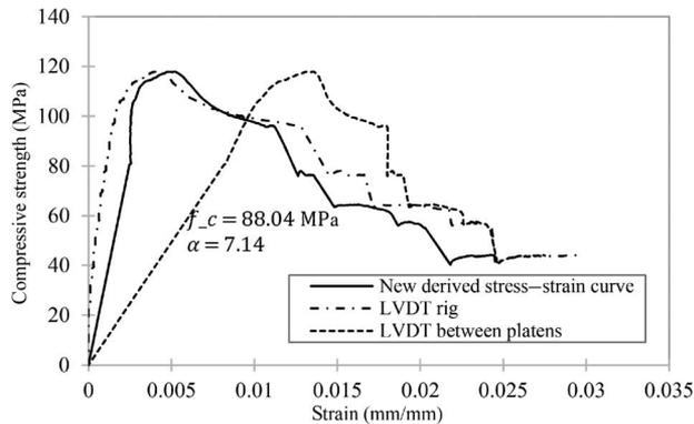
the correction factor. However, the correction factor would vary depending on the type of testing machine, the method of specimen preparation, the loading pace, loading patterns, and the overall testing procedure.
