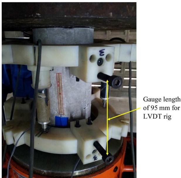
FIG. 8 Location of LVDT between machine platens.
