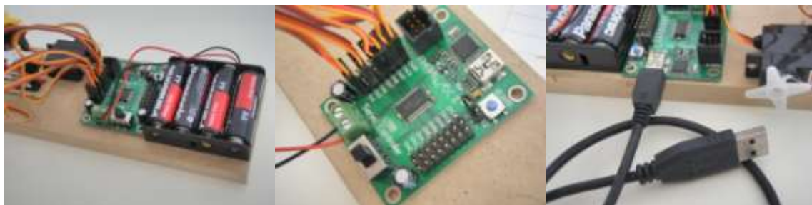
Figure 3. Mounting of the controller unit in the forearm of the gripper.
